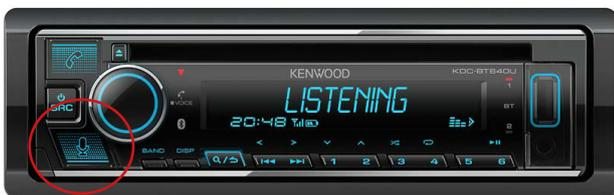
12. Press the **[MICROPHONE]** button on the KDC-BT640U
