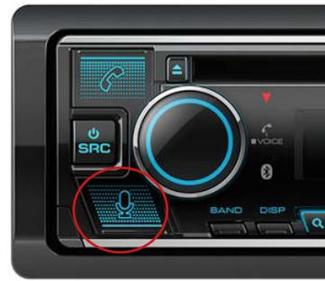
7. Then press the **[MICROPHONE]** button on the KDC-BT640U
