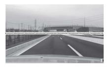
2. Press the [MENU/OK] button, use the [▲]/[▼] buttons to align the guideline with the horizon, and then press the [MENU/OK].
