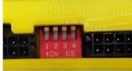
Dip Switch 1 OFF = Low Resolution (480 x 240) Golf
