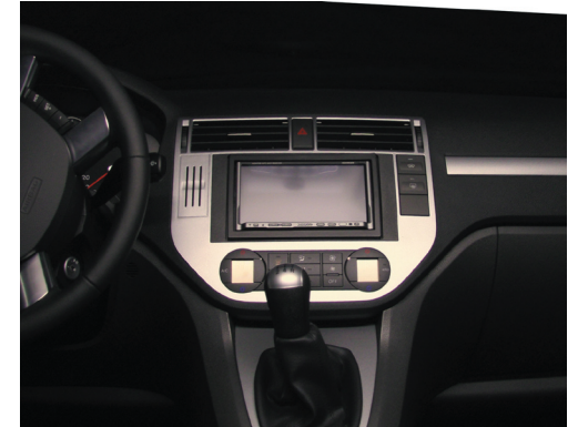
Place head unit and radio trim
