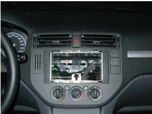
Place 2-DIN metal bracket
