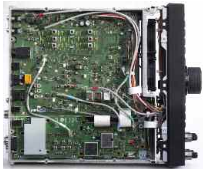
PHOTO 3: Underneath view showing signal processing boards.
