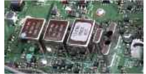
PHOTO 6: 2nd IF roofing filters.
