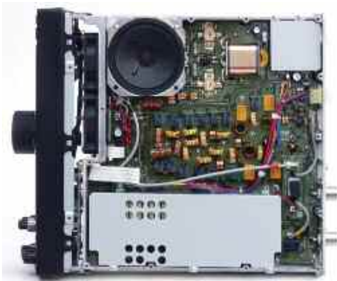
PHOTO 2: Top view with covers removed showing PA, output filters and auto ATU.
